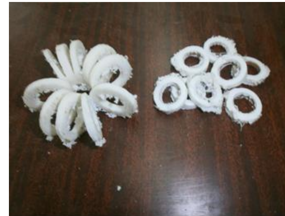
Figure 2. Polyvinyl chloride pipe trimmings
