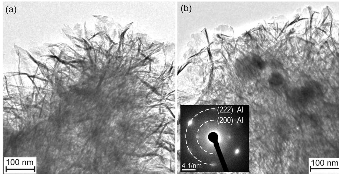
**Figure 3.** TEM micrographs of Al oxyhydroxide before (a) and after (b) microwave irradiation; an electron diffraction pattern is shown in the insert
