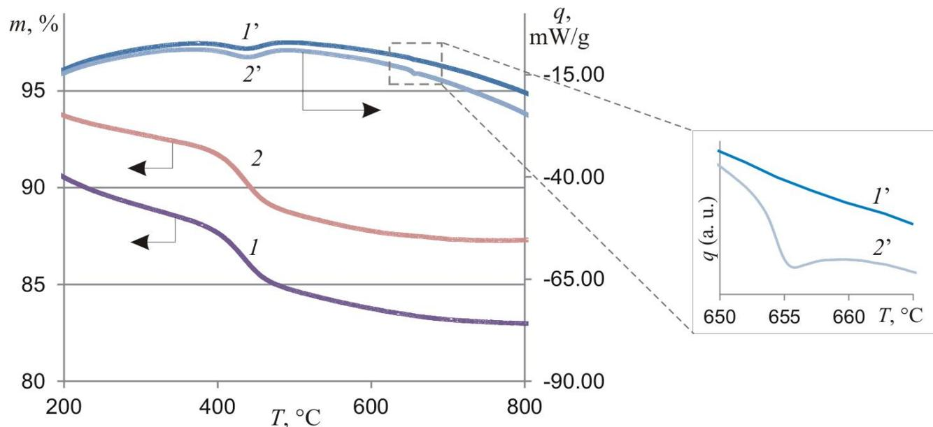
**Figure 1.** The TG (1,2) and DTA (1',2') curves of linear heating of the Al oxyhydroxide samples before (1, 1') and after (2, 2') exposure to the powerful short-pulse microwave radiation; in the insert on the right, the parts of DTA-curves corresponding to the temperature area of Al melting are shown
