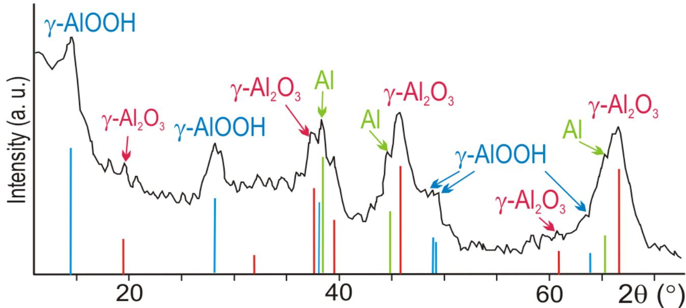
**Figure 2.** XRD-pattern of Al oxyhydroxide exposed to microwave radiation for 3 min under ambient conditions
