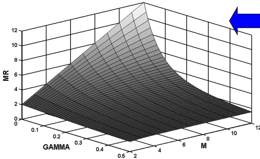
**Dependency between function  $M_R$  and  $\gamma$  parameter for BEJs with different number of layers ( $M$ ). A parameter,  $\gamma$  characterizes a ratio of the fretting wear cyclic rate to the microcrack growth cyclic rate.**
