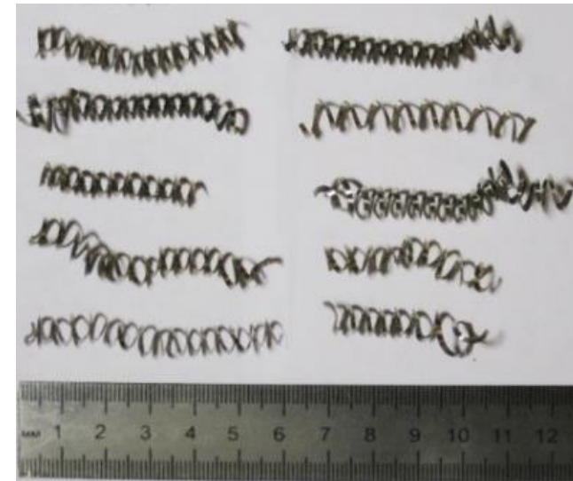
cutting with vibrations A = 5 - 10 microns; f = 5 - 10 Hz
