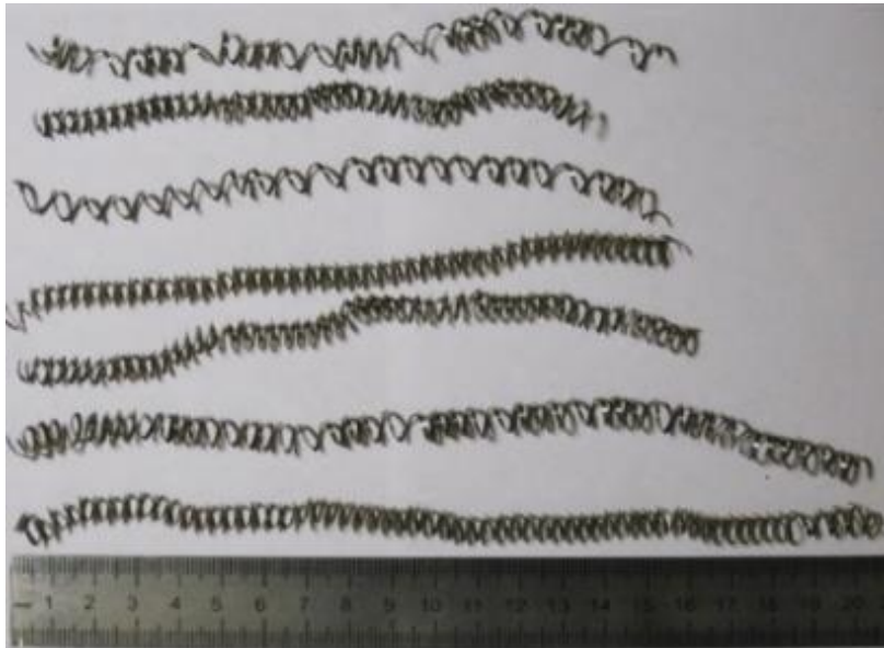
traditional turning cutting speed of 85 m/min; feed of 0,26 mm/rev
