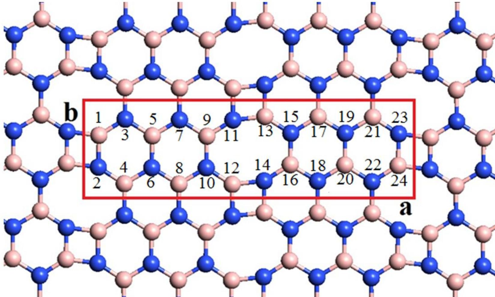
Figure 1. Geometrically optimized structure of 4-6-8e boron nitride layer and its unit cell with indication of atomic numbering (boron atoms are shown in beige, nitrogen - in blue).
