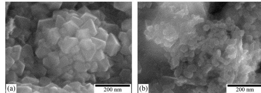
Samples of nanocomposites on the steel surface obtained in the presence of PVP (a) and PEGML (b).
