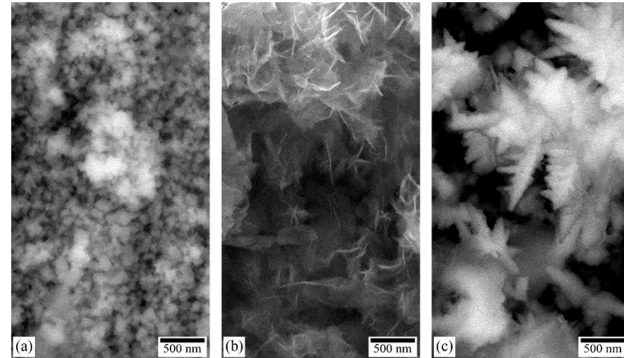
SEM-images of samples obtained in the presence of PVP (a), PEGML (b), PEG (c).
