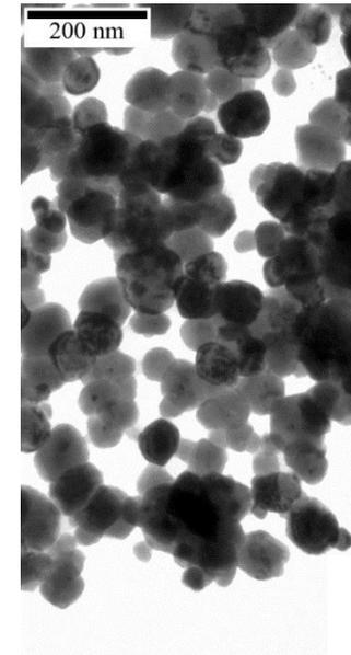
Sol particles formed as a result of ultrasonic treatment of the reaction system during the formation of samples in the presence of PVP 360000. It was noted that sols were not formed in the absence of PVP.
