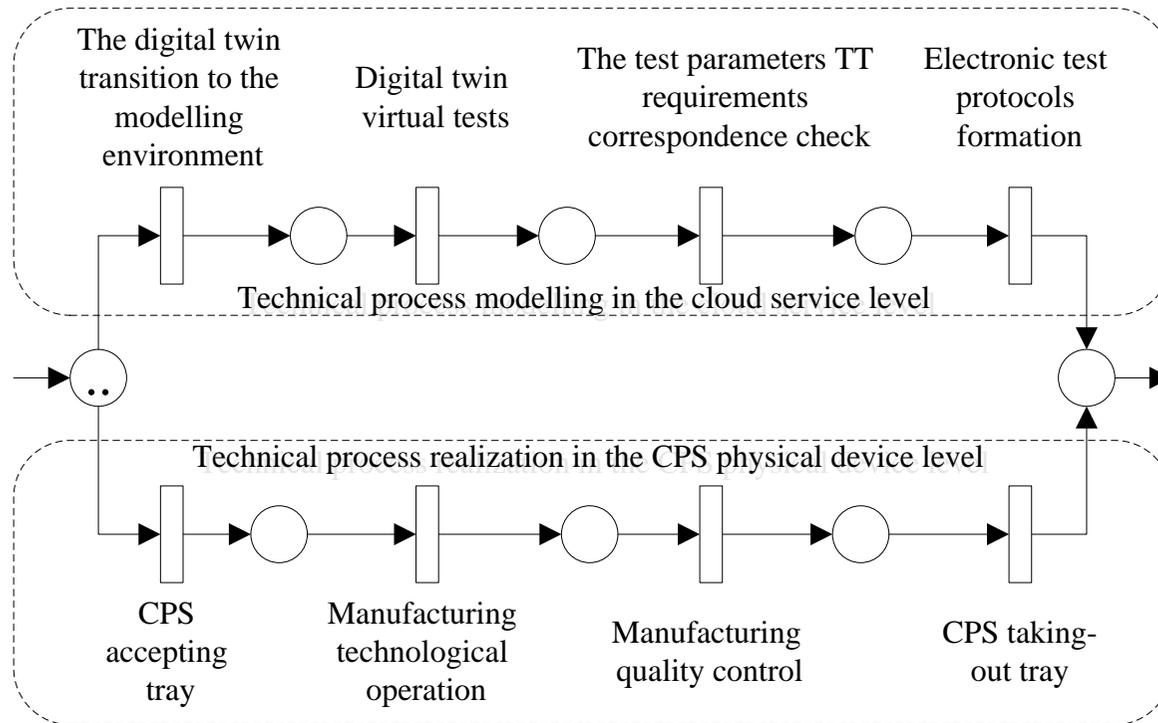
**Figure 3.** A Petri net scheme to describe the Industry 4.0 cyber and physical system operation.
