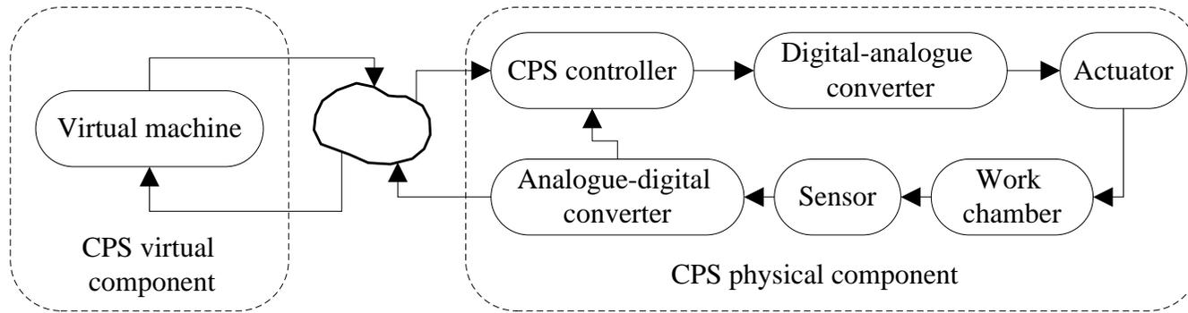
**Figure 1.** Cyber and physical system functioning scheme as an automatic control digital system.
