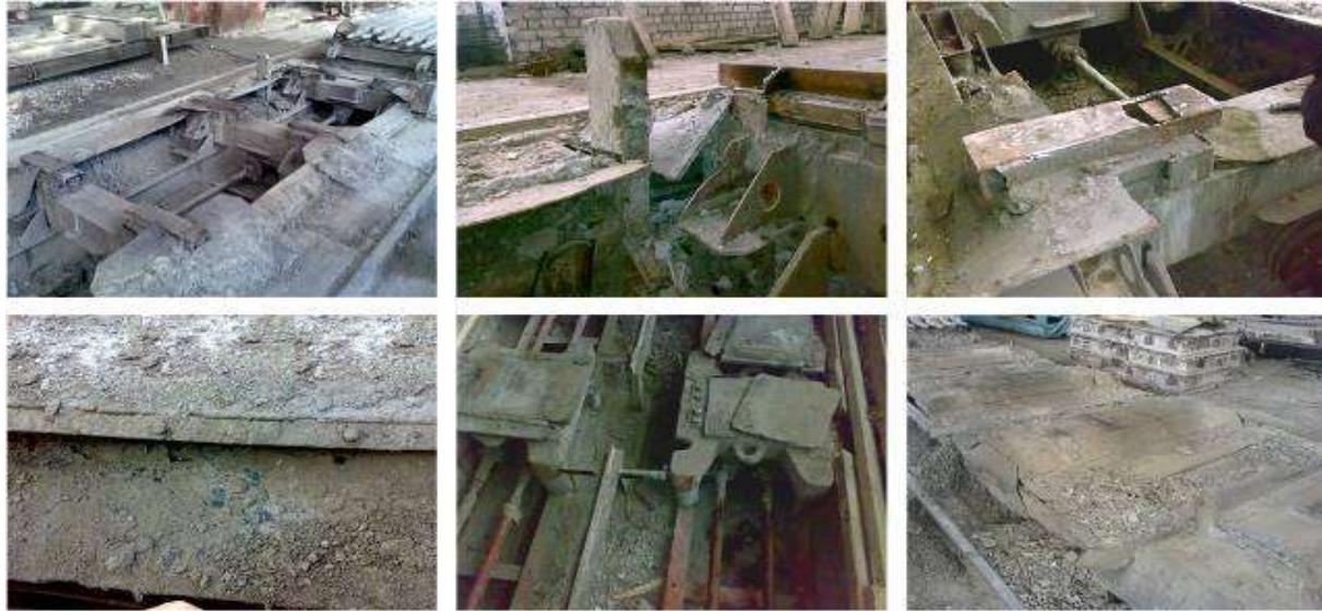
Figure 1. Photo-fixation of failures of working bodies of vibrating platforms
