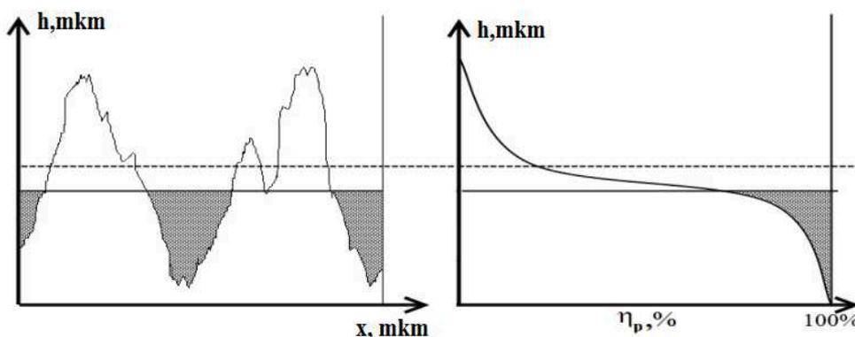
Fig. 1. Procedure of determining volume of voids of rough layer
