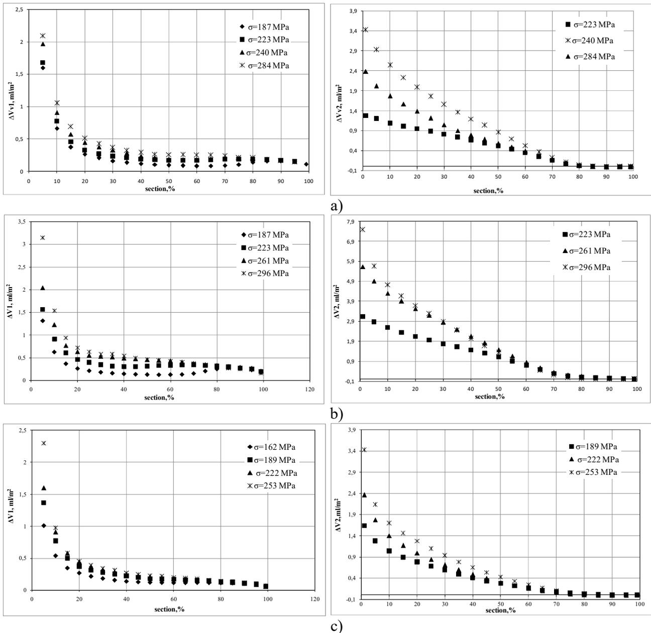
Fig. 5. Change of void volume in layer-by-layer sections at different pressures in deformation zone and at different roughness of roll a)  $R_a=4.2 \mu\text{m}$ ;  $R_{Pc}=58 \text{ 1/cm}$ ; b)  $R_a=5.03 \mu\text{m}$ ;  $R_{Pc}=54 \text{ 1/cm}$ ; c)  $R_a=8.3 \mu\text{m}$ ;  $R_{Pc}=37 \text{ 1/cm}$ .
