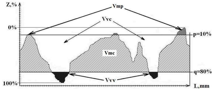
Fig. 2. 3D volume characteristics of rough surface layers
