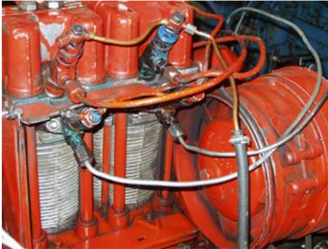
Figure 2. Nozzles for supplying methanol (installed at the top) and diesel fuel (installed at the bottom)
