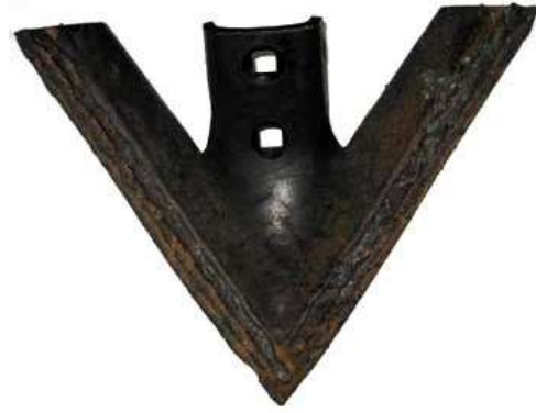
Fig. 1. Cultivator blade, reconditioned by surfacing
