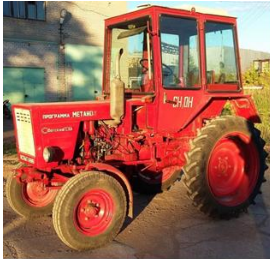
General view of the T-25A tractor with a power system modernized for methanol with a dual combustible supply system
