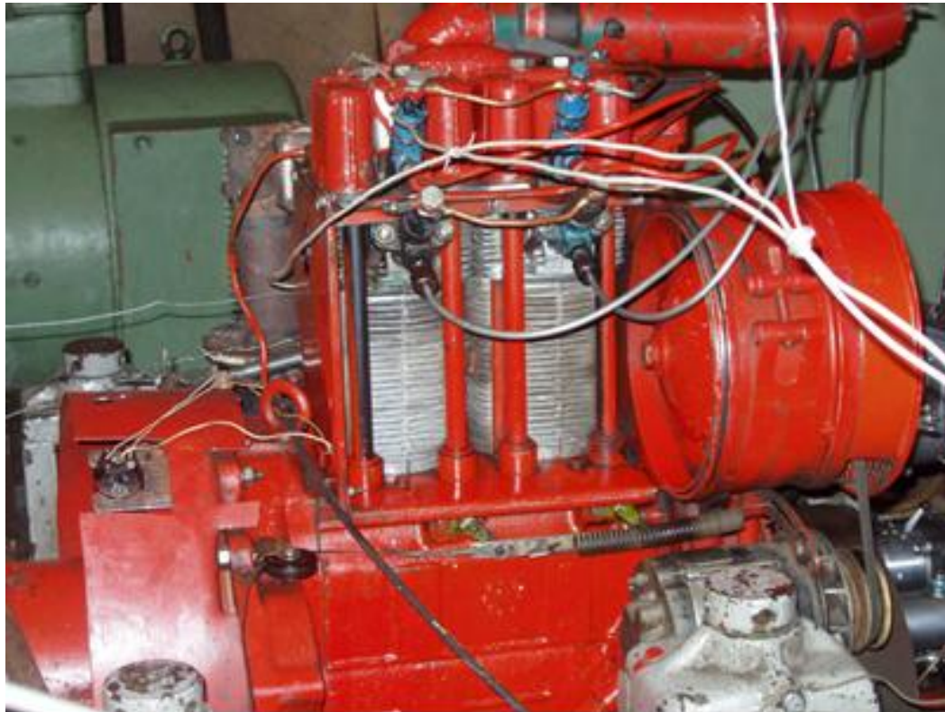
View of the nozzles for supplying methanol (installed at the top) and diesel combustibile (installed at the bottom) of a motor 2H 10.5 / 12.0
