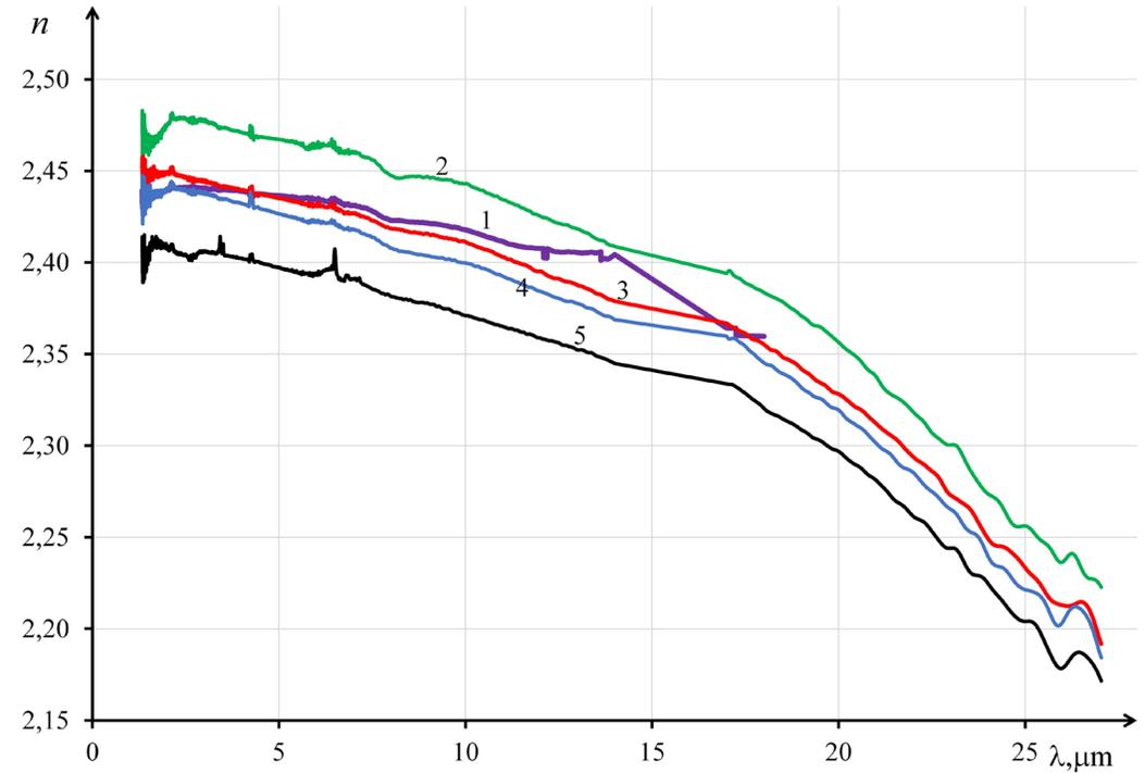
**Figure 2.** Dispersion of the ZnSe refractive index (1 - according to the RT spectrum of the plate, 2-5 according to the R spectra from the surface)
