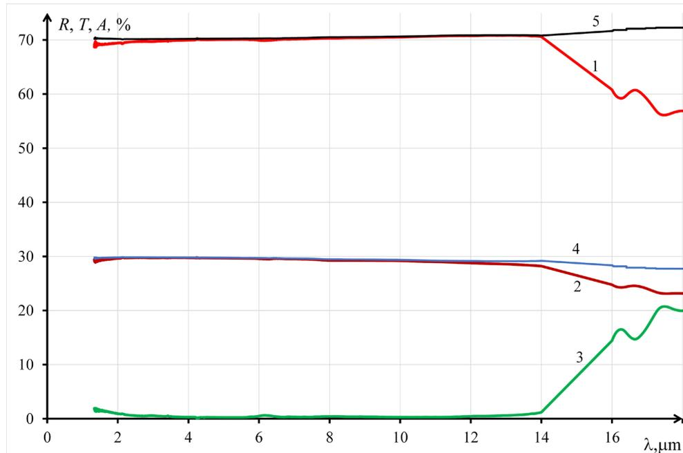
**Figure 3.** ZnSe plate spectra (1 - experimental transmittance spectrum, 2 - experimental reflection spectrum, 3 - experimental absorption spectrum, 4 - corrected reflection spectrum, 5 - corrected transmittance spectrum)
