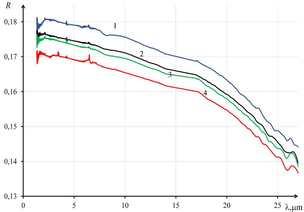
**Figure 1.** 1,2,3,4 -  $R_S$  reflection spectra from the surfaces of four samples of zinc selenide
