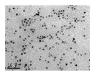
A copper-containing sol was formed by reduction by tert-butylamine-borane in the presence of poly-N-vinylpyrrolidone. The dispersed phase of a sol is actually a nanocomposite that includes nanoparticles (3-12 nm in diameter) and macromolecules.
