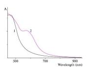
Electron spectroscopy studies have shown that sols containing Cu<sub>2</sub>O particles (1) or Cu particles (2) are formed.
