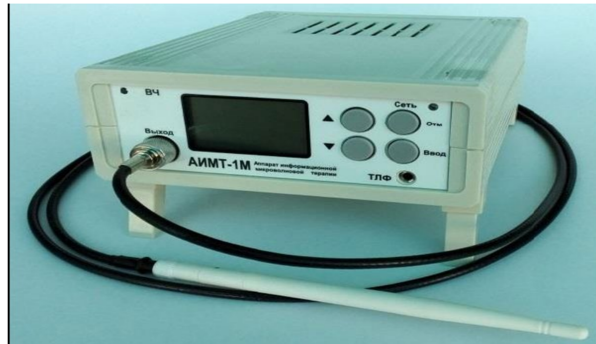
Figure 2. Device for simulating solar microwave radiation (AIMT-1) in the frequency range (4.0-4.3) GHz
