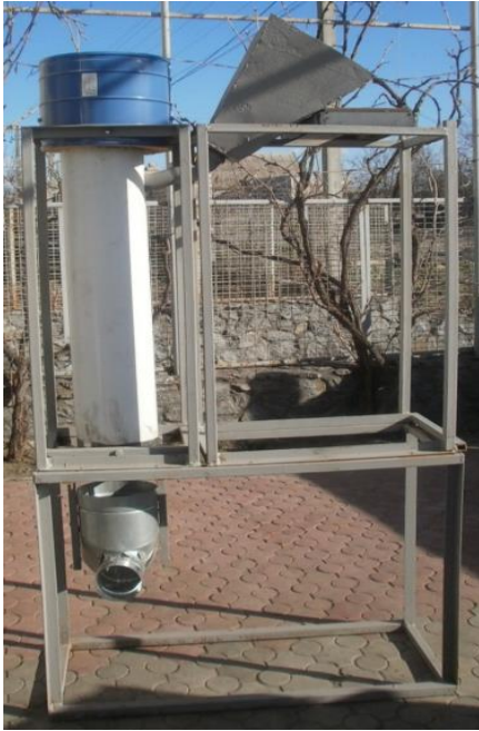
Figure 1. Experimental model of the developed vibroaspiration seed separator
